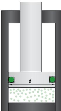
Bore sealed gas springs are ideal for small movements and very strong forces with a maximum contact pressure.
