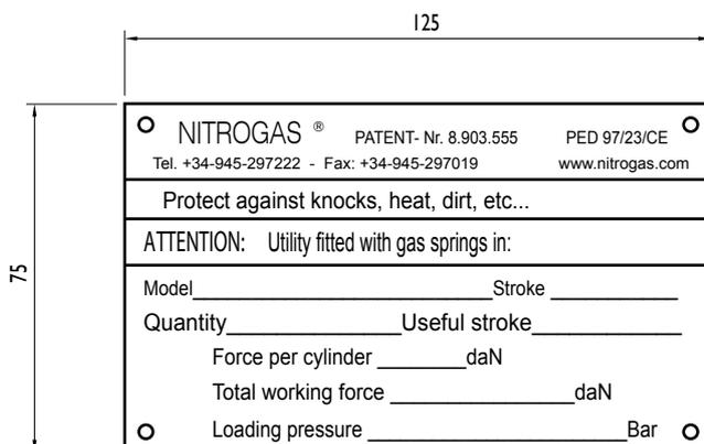
NITROGAS recommends identifying tools containing high pressure nitrogen gas springs to ensure the proper handling of the gas springs.
