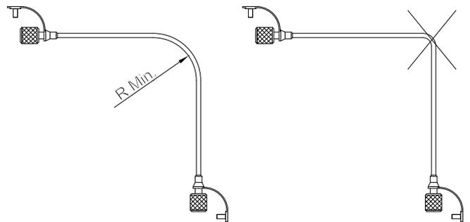
5. Fix the hose correctly to avoid mechanical damage. We recommend using RM-108 clips to fix the hose.
