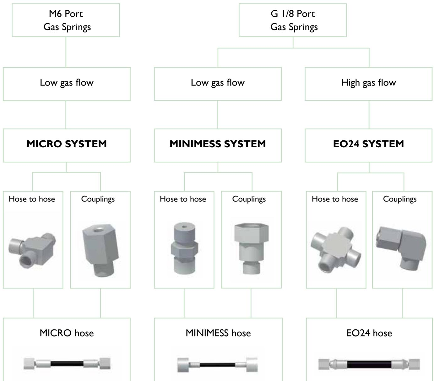
The possibility of being or not connecting, as well as the connection type (M6 or G1/8") of each gas spring model is indicated in the specification sheet of each model.
