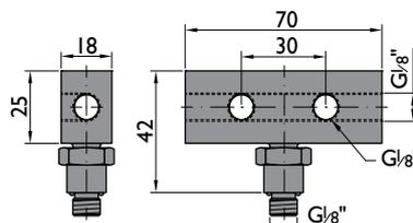
\* Includes a non-return valve to keep the pressure on each gas spring individually when removing the hoses.
